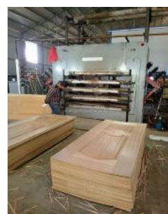
Fig (43) The usage of compressed straw panels as doors [46].
