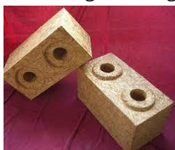
Fig (38) Lego Blocks from Straw [41].
