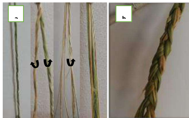
FIG. 11: ROPES MANUFACTURING A) TWINNING PROCESS B)
