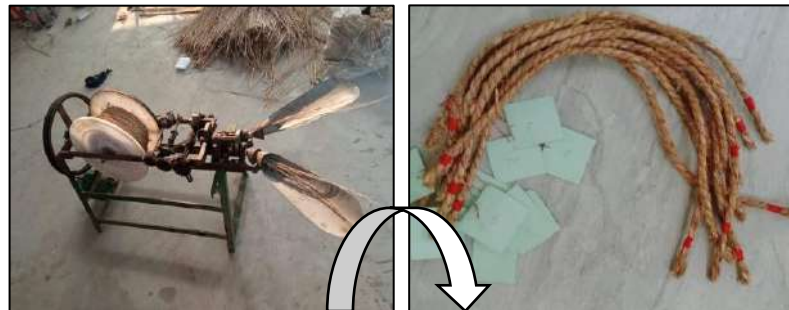
Fig. 4: BRRl( Bangladesh Rice Research Institute ) straw rope maker: The BRRl straw rope maker was fabricated in a research workshop to twist straw into rope and increase the versatile use of a straw.
