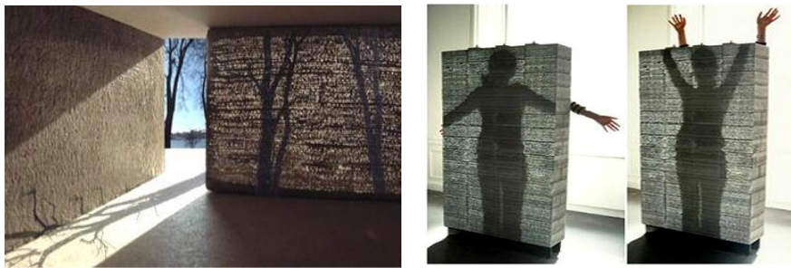
Figure (21) shows light-permeable concrete and its importance in creating connection with the surrounding environment
