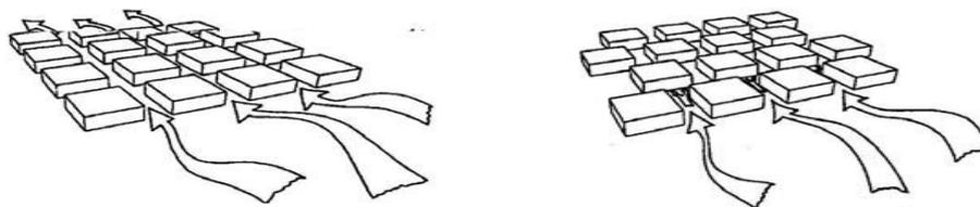
**Fig. 1. The airflow inside the city, right in the case of parallel and straight streets, left in the case of narrow and winding streets (Nastaran January 2013).**
