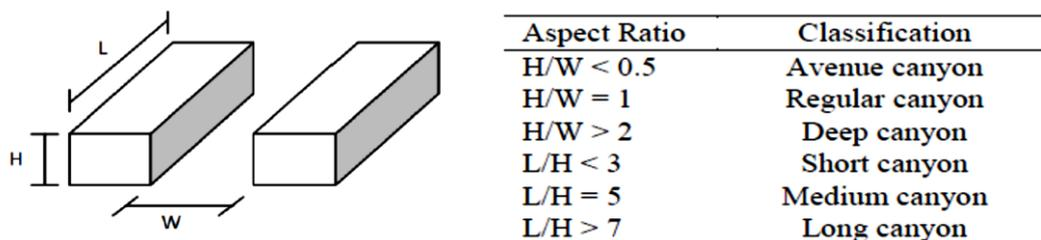
**Fig. 3.** Classification of canyons and their geometric shape according to buildings (Afiq W.M.Y.1,Azwadi C.S.N, Saqr,K.M. september 2012).
