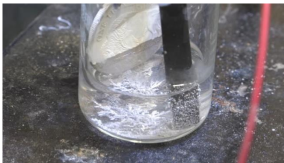
Figure5. the cathode just starts to bubble hydrogen
