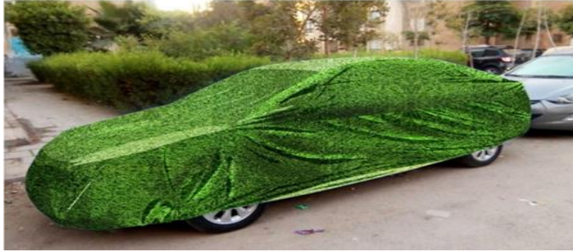
A) Printed cover made of glass fibers and nylon.
