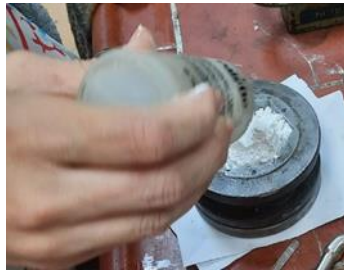
shape no. 9 shows the addition of the polyvinyl alcohol (7%)
