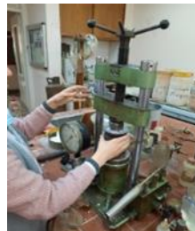
shape no. 10 shows placing the mold inside the hydraulic presser
