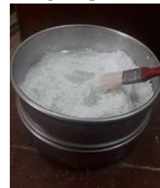
shape no. 6 shows glass powder sift.
