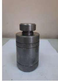
shape no. 8 shows a rounded iron model used in pressing the samples
