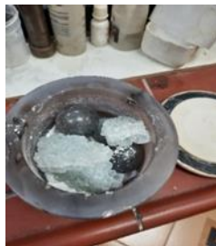
shape no. 4 shows broken glass in the glass grinder before its activation
