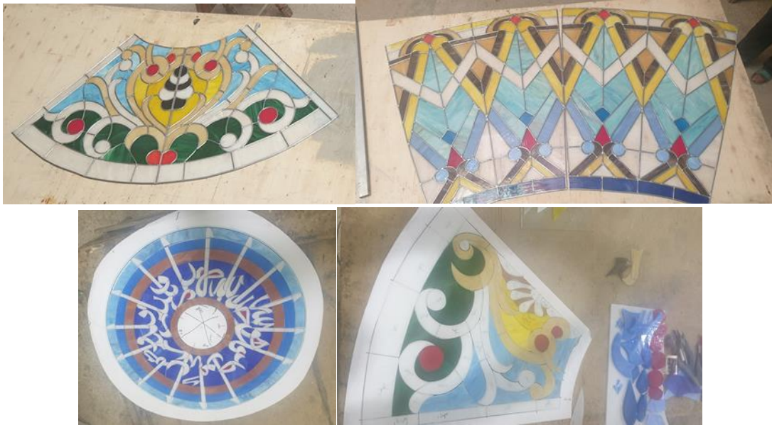
Shape 27 clarifies the process of cutting and mesh the dome glass according to the design Glass was collected and interlocked with colored opal opaque glass according to the suggested design and executive drawing that was done previously is being applied on the required measures, then the dovetailing process and mantling of glass through lead sticks then welding with tin then cementation or pasting and oxidation, in order to get the colored, dovetailed required piece of glass.
