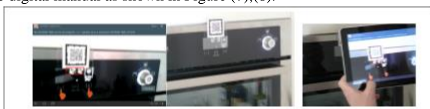
a b c A - Oven with Vuforia frame marker pen and QR code attachment B - GuideMe highlights the corresponding operating elements C - Screenshot from GuideMe with featured launch items Figure (6/a,b,c) shows the GuideMe prototype in action
