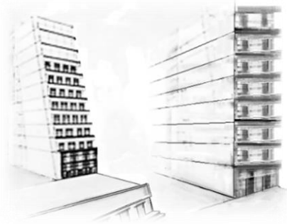
Figure No. (2) Shows a building built according to the requirements of Law 119 of 2008, and the other has a gradation of duty to be followed in modern licenses to ensure that adjacent and opposite neighbors enjoy natural resources to provide a good healthy environment.
