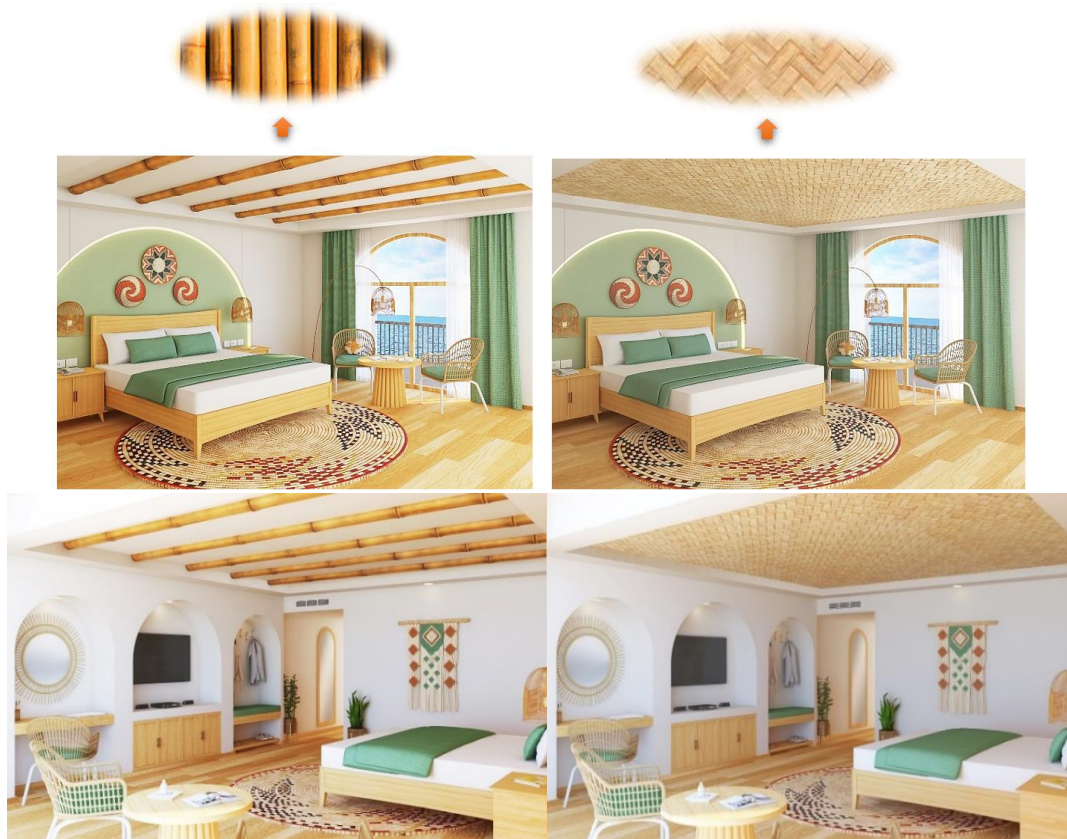
(Figure 33 ) Two designs for the ceiling of the room using bamboo material.
