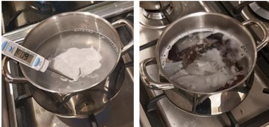
Figure (20) Dimensional stability after washing test at 60°C
