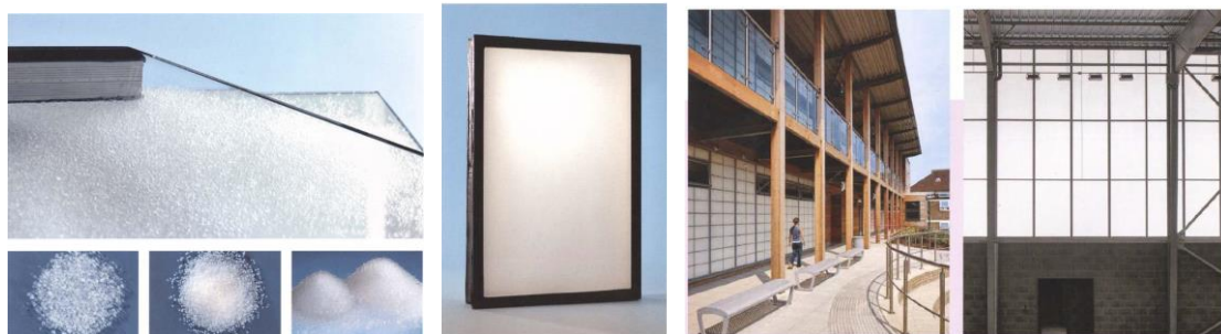
Fig. 15, show the translucent nanogel granulate, the use of aerogel in the windows in School extension, London, England [1]
