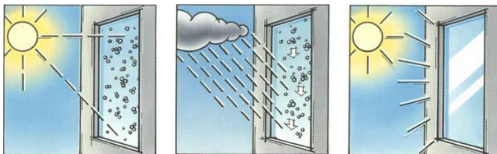
Fig. 9, show organic dirt and grime is broken down and "decomposed". UV light, present in sunlight, is necessary to initiate photocatalysis. When water impacts on the surface, it spreads to form a film washing away the loose dirt. [6].
