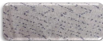
FIGURE [15] SAMPLE [10] USING TWILL STRUCTURE WITH COTTON WEFT KNOP
