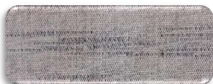
FIGURE [12] SAMPLE [7] USING BASKET STRUCTURE WITH COTTON WEFT SLUB
