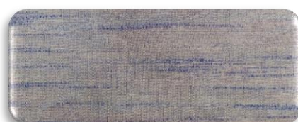
FIGURE [13]SAMPLE [8] USING BASKET STRUCTURE WITH POLYESTER WEFT SLUB
