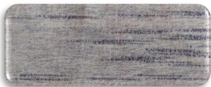
FIGURE [6] SAMPLE [1] USING TWILL STRUCTURE WITH COTTON WEFT SLUB
