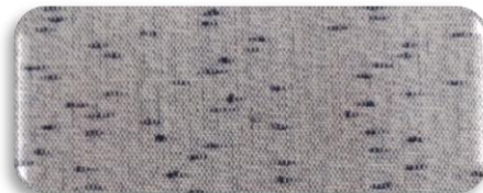
FIGURE [21] SAMPLE [16] USING MATT STRUCTURE WITH COTTON WEFT KNOP
