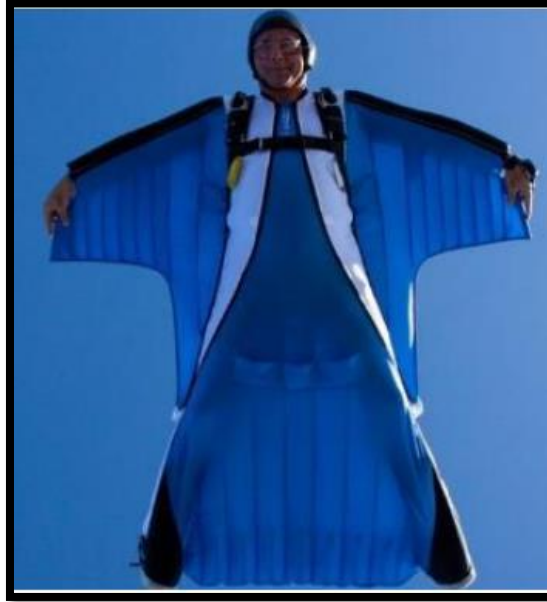
FIGURE 19: INTERMEDIATE WINGSUIT WITH INCREASED ARM WING SIZE, END OF ARM WING GRIPPERS, AND AN EXTENSION OF THE ARM-WING DOWN THE LEG OF THE PILOT (TONYSUITS 2010)
