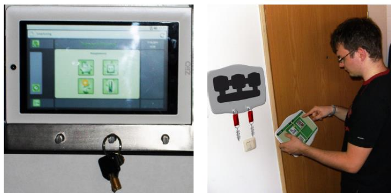
Figure (5). An interactive key holder tool used as part of behavioral change motivation techniques, to inform people about their energy-consuming devices to enable them to act. Source: Rist. et al. 2012.
