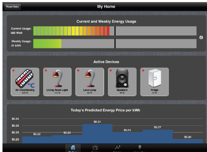
Figure (3). An example of a metric visualization used in a USEM mobile app to display current and power consumption data (top). Source: Reinhart. et al. 2014.
