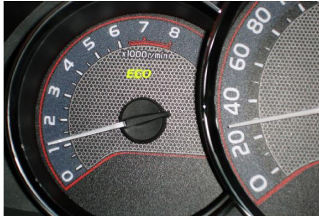
Fig (4). Example of a car dashboard with the "ECO" indicator, indicating whether the driving mode is economical or not.
