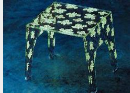
Picture No. (2) shows one of the glass chairs that was covered with a glass-ceramic phosphorescent material.
