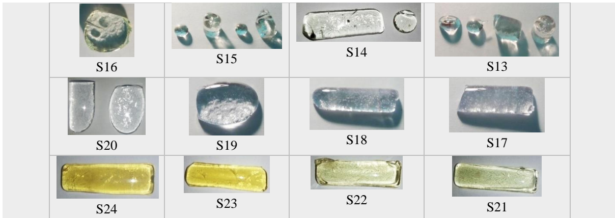
Picture No. (6) shows the shape of the glass samples for the first group after completing the cooling process according to their chemical composition
