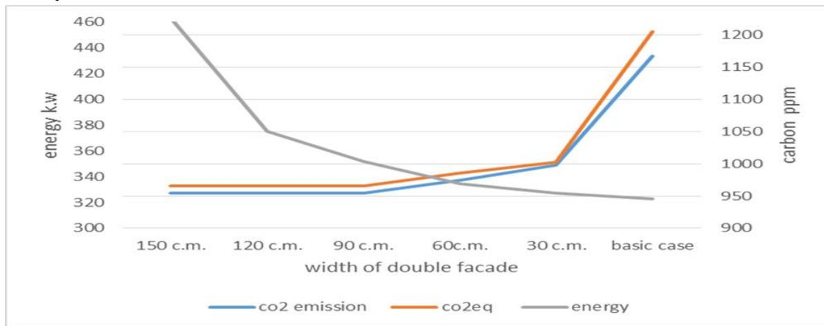
Fig. 4 Results of simulation CASE1: the use of box window facades
