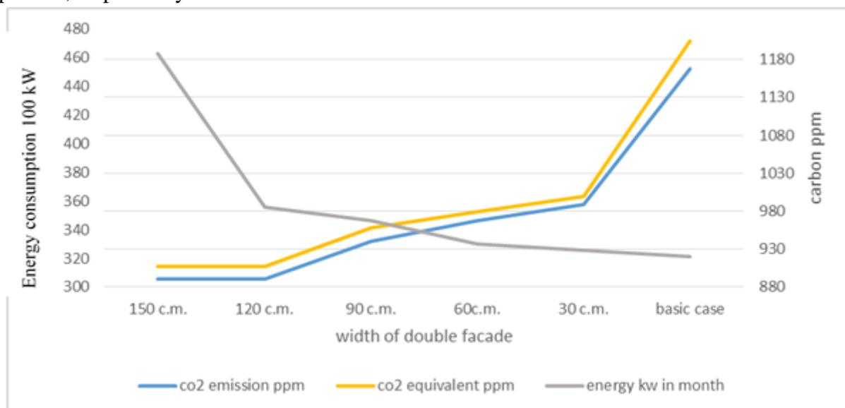
**Fig. 5 Results of simulation CASE 2: the utilization of corridor façades**
