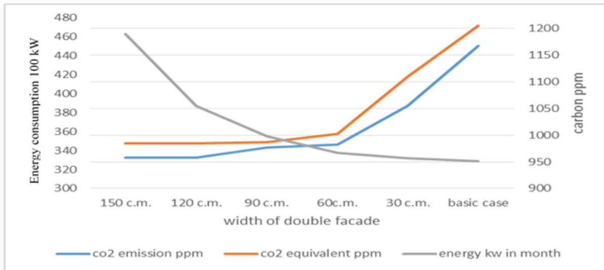
**Fig. 6 Results of simulation Case 3: The employment of Shaft box facades**
