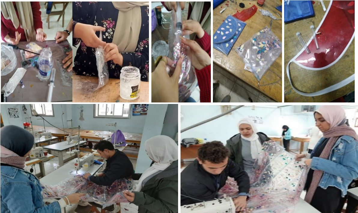
Figure (19) Steps of how using the gel between the dress and accessories layers, then sewing the different parts together
