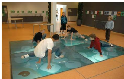
Figure (5) Interactive floors consisting of tiles, under which sensors are installed to interact with human movement
