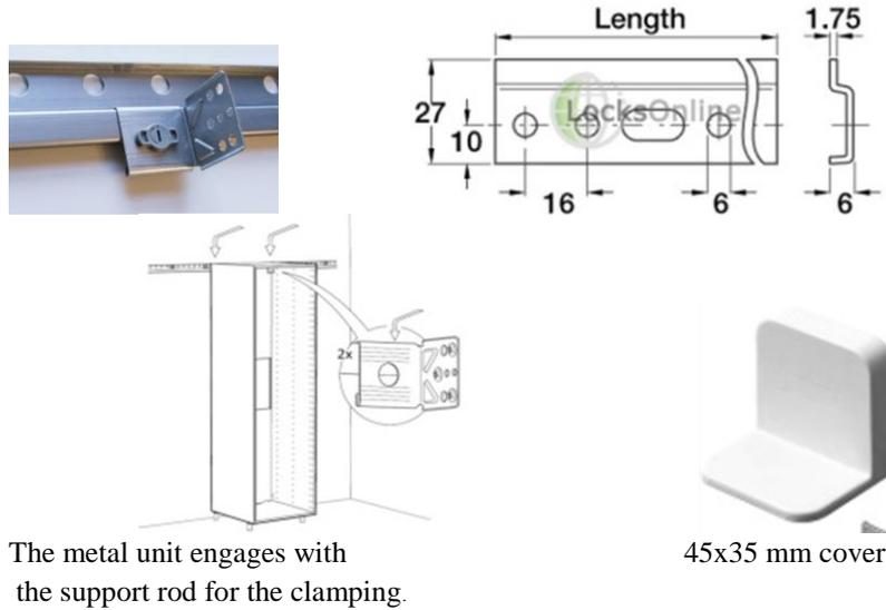
**Fig.1: Dimensions of metal hung to attach the hanging cases to the object of the cheese.**
