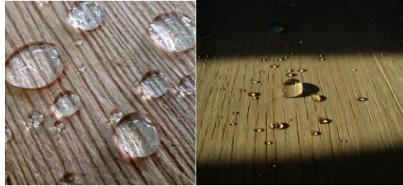
Figure (5) shows the Nano-treated wood, which is characterized by its resistance to water leakage into its fibers
