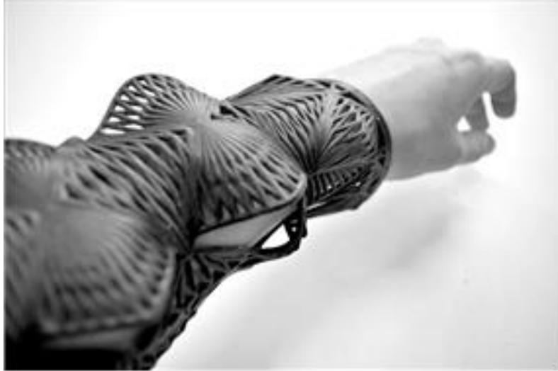
Picture 4: Body Activated Sleeve equipped with sensors to map people's motions
