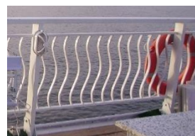
Figure (1) Fences on weather decks
