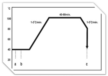
Figure (2) Dyeing curve of Acidic dye.
