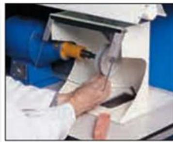
5-Mechanical processes are used in finishing gold jewelry to significantly reduce manpower and reduce production costs compared to laser finishing operations. Different types of finishing equipment and media can be used in the mechanical process, and are selected according to the type of product to be completed.
