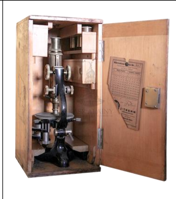
(12) A lacquered brass microscope by J.Thamm A.G Berlin circa 1926. Rack and pinion focusing with fine adjustment over a rotating stage and concave mirror also including 2 spare eye pieces marked (4) and(5) and three lacquered brass objectives cases with fitted mahogany case.J.Thamm, Berlin,N.W,Karl Strasse,Berlin, Germany.
