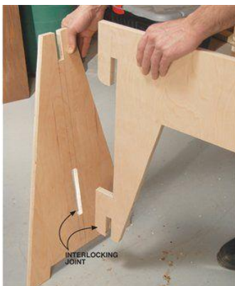
Figure (16) shows the formation of wooden pieces using digital control technology, which ensures the accuracy of the installation
