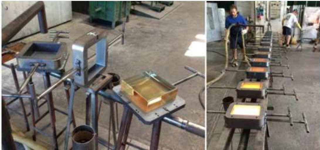
Figure (4) shows the method of pouring the solid glass block inside the mold
