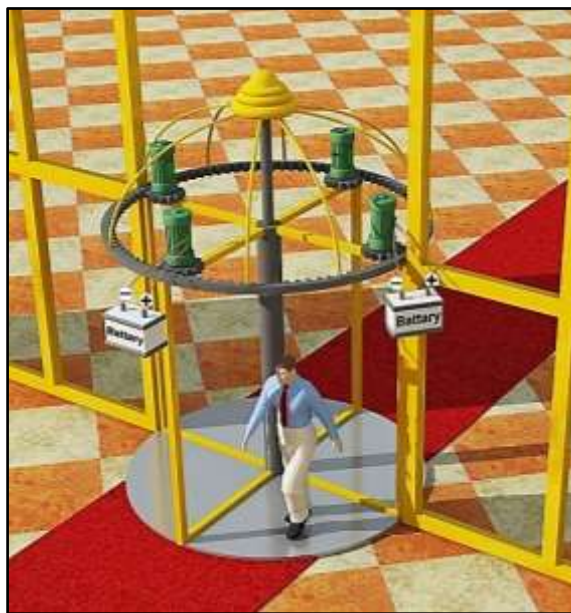
Fig (10) shows how to use the revolving door in power generation
