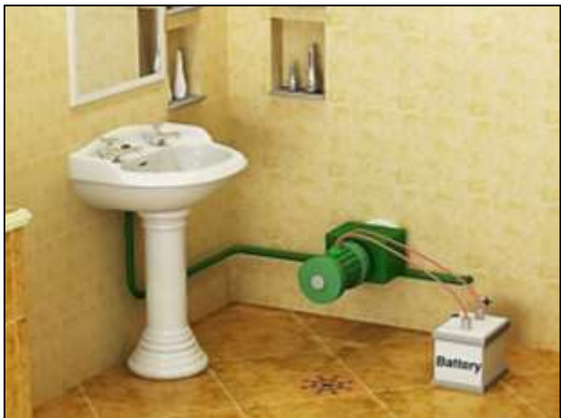
Fig (8) shows the unit installed on the water pipes with fan blades, gearbox and power generator
