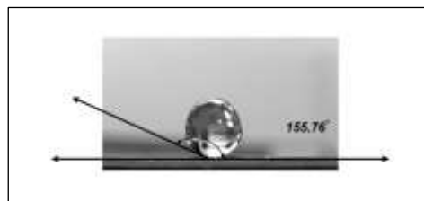
Figure 15 Contact angel before treatment Figure 16 Contact angel after treatment
