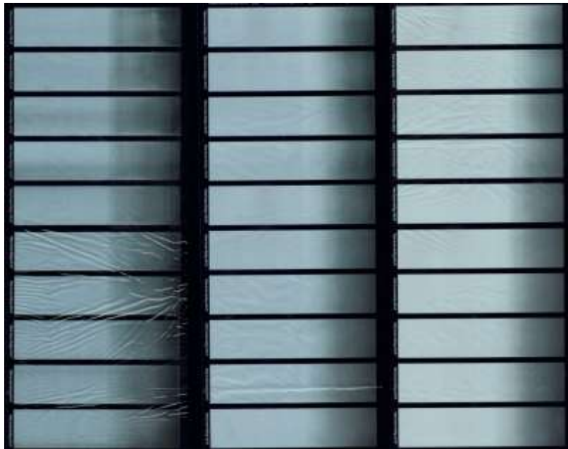
Figure (6) Visual Appearance of First Test Target Printed using 3 different anilox rolls
