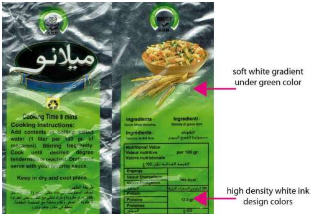
Figure (1) rotogravure sample shows soft white gradient and high white ink density at the same time
