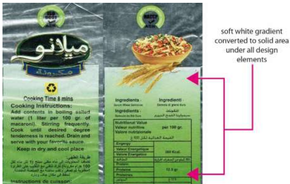
Figure (2) Flexography sample shows white gradient conversion to solid area under the design elements
