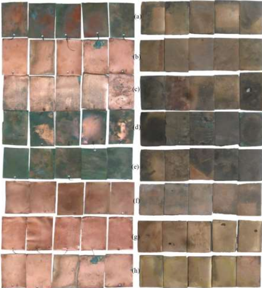
Fig.17. Treated coupons after climate chamber test with Cl (right) and SO 2 (left) a- mic., b- NaC 10 ., c- BTA., d- Cys., e- unt., f- Met., g- Par., h-ATA.
