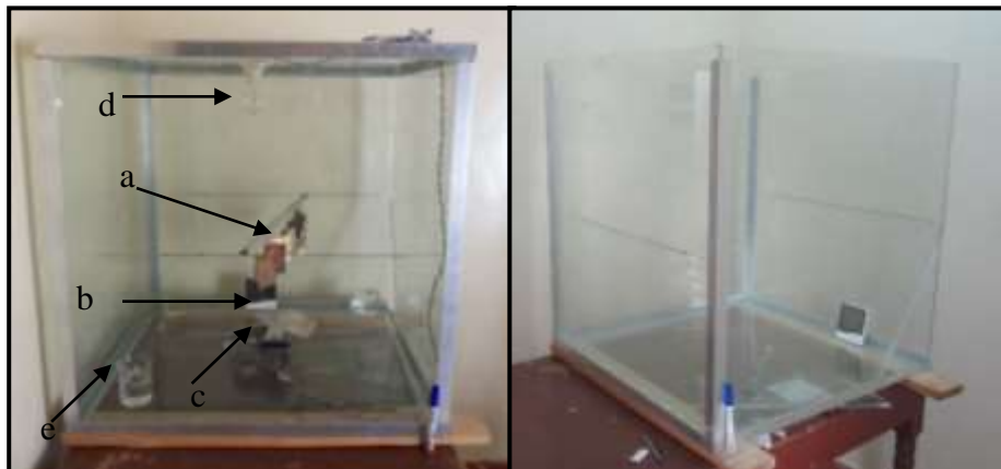
Fig. 2. Chamber used to accelerated corrosion during and before manufacturing stage, a: coupons suspended in the middle of the chamber. b, an instrument used for measuring the moisture. c, fan to mix the gas with the air inside the room, d, electric lamp to raise the temperature if necessary, e, the saturated solution to adjust the humidity.
